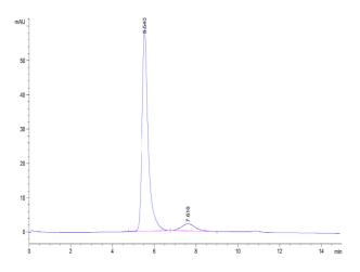
The purity of Human LTBR is greater than 90% as determined by SEC-HPLC.
