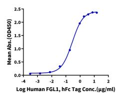
Immobilized Human LAG3, His Tag at  $5\mu g/ml$  (100 $\mu l/Well$ ) on the plate. Dose response curve for Human FGL1, hFc Tag with the EC50 of 0.28 $\mu g/ml$  determined by ELISA.
